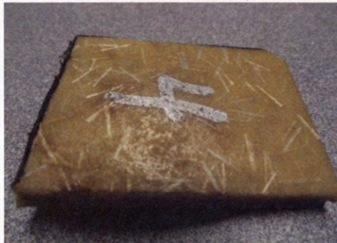
(c) Polyurea B with Discrete E-glass Fibers
