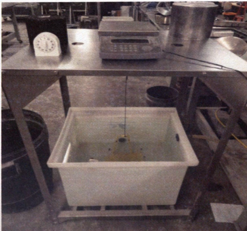
Figure 3.16 – Water Bath Setup for Density
