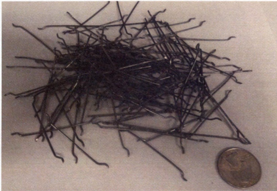
Figure 3.4 – Propex Novocon 1050H Steel Fiber
