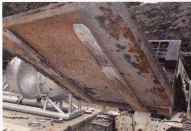
(g) Bulge in Tension Face
